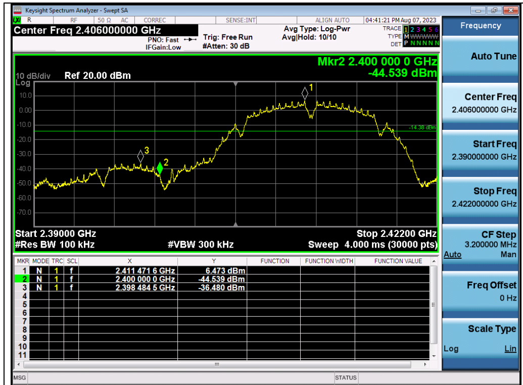
Test_Graph_802.11b_ANT1_2412_1Mbps_Lower Band Edge Emissions
