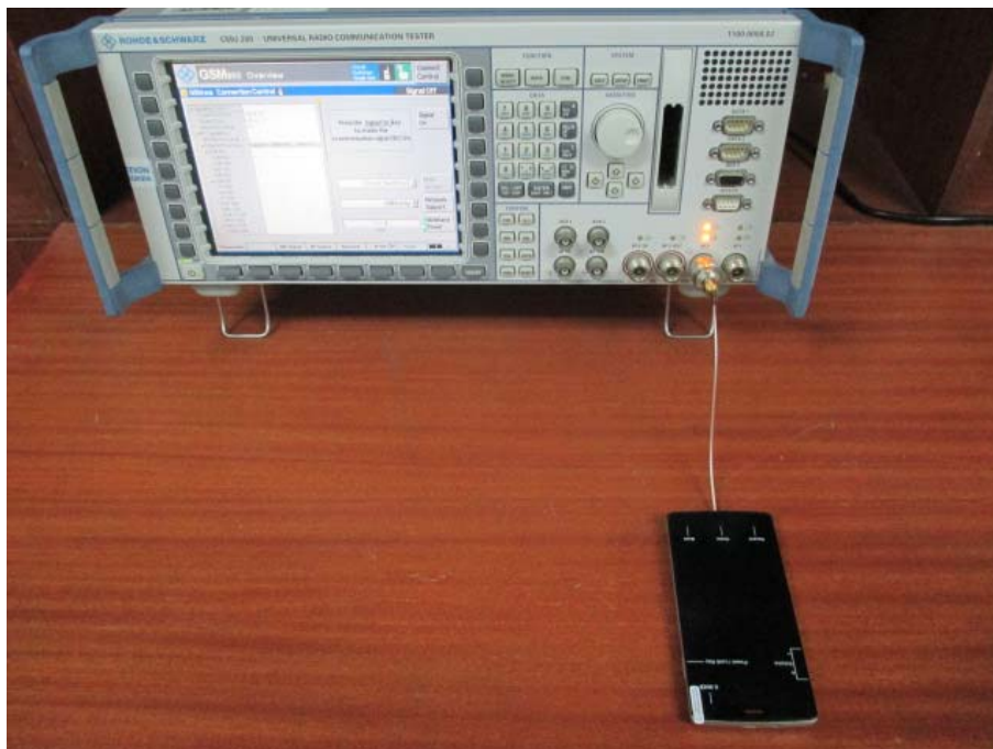
Photograph –2G&3G Conducted Test Setup
