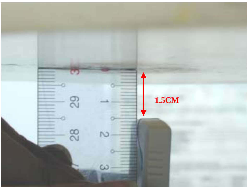
Fig.8 Photograph of the antenna tip is upward and at a distance of 1.5 cm from the base of the phantom.
