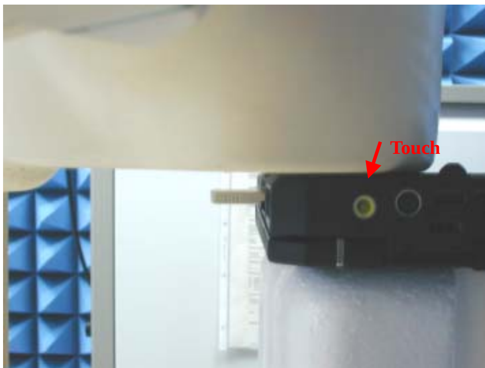
Fig.4 Photograph of the Bottom of the Pc is paralleled and at a distance of 0.0 cm from the base of the phantom.
