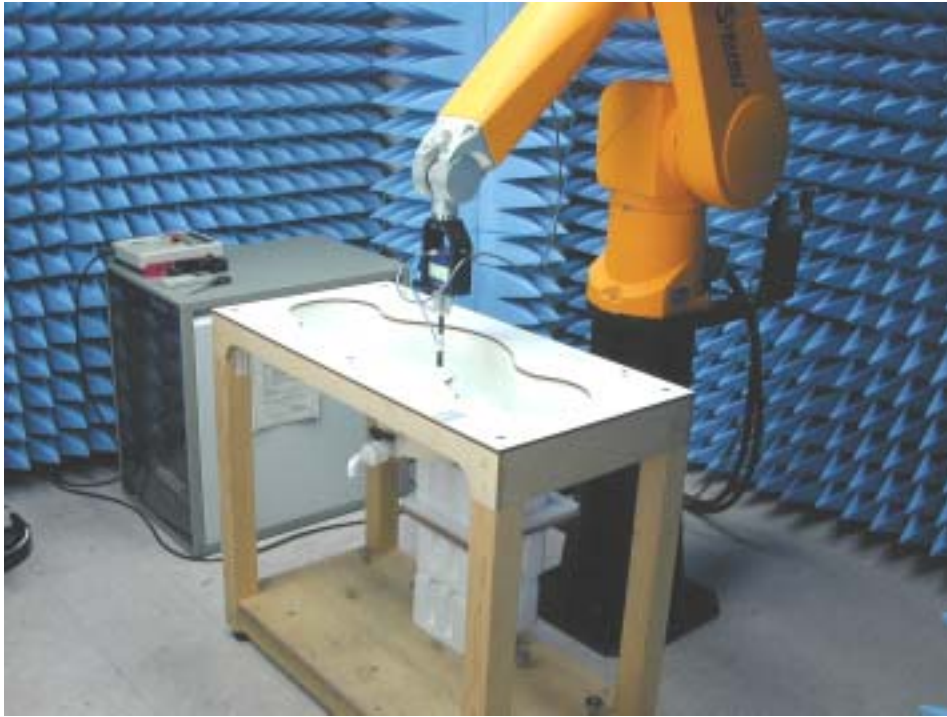
Fig.1 Photograph of the SAR measurement System
