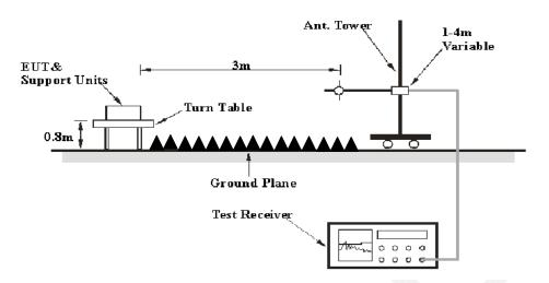
The radiated emission tests were performed in the 3 meters chamber test site, using the setup accordance with the ANSI C63.4-2009. The specification used was the FCC Part 15.109 Class B limits.
