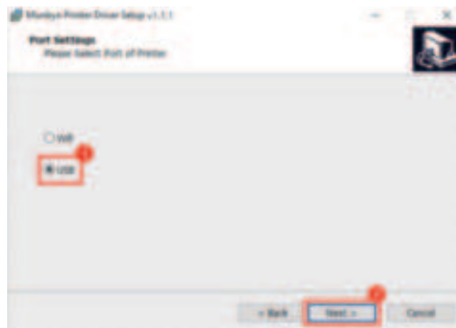
Figure 3-3 Select USB Port for Installation
