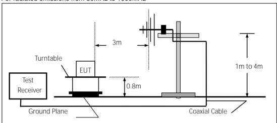
(c) For radiated emissions above 1000MHz
