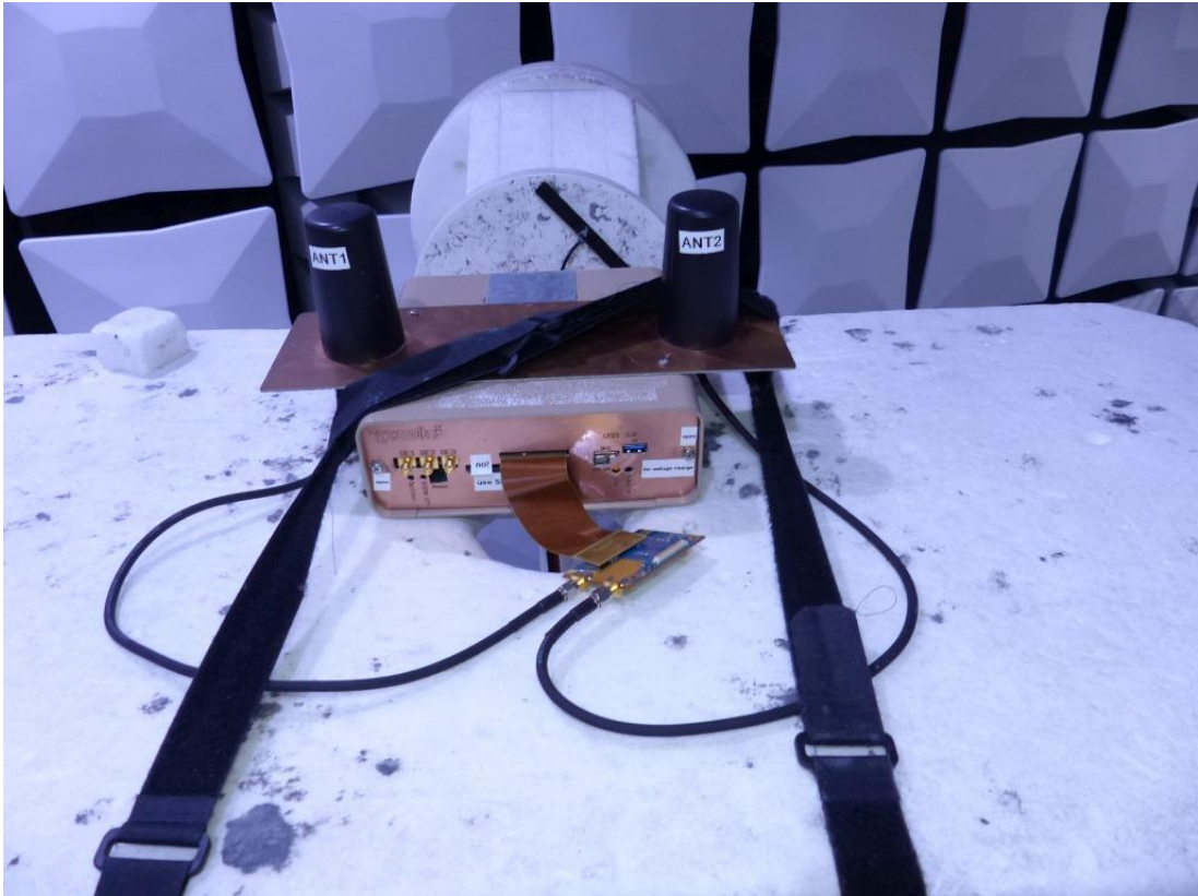
Photo 4: Test setup for radiated measurements (Enclosure, fully-anechoic chamber, 1-18 GHz intentional radiator §15 / 30 MHz – 10/20 GHz §22/24/27)
