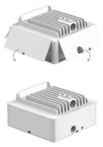
Step 9: Use four screws to securely affix the side covers to the enclosure.
