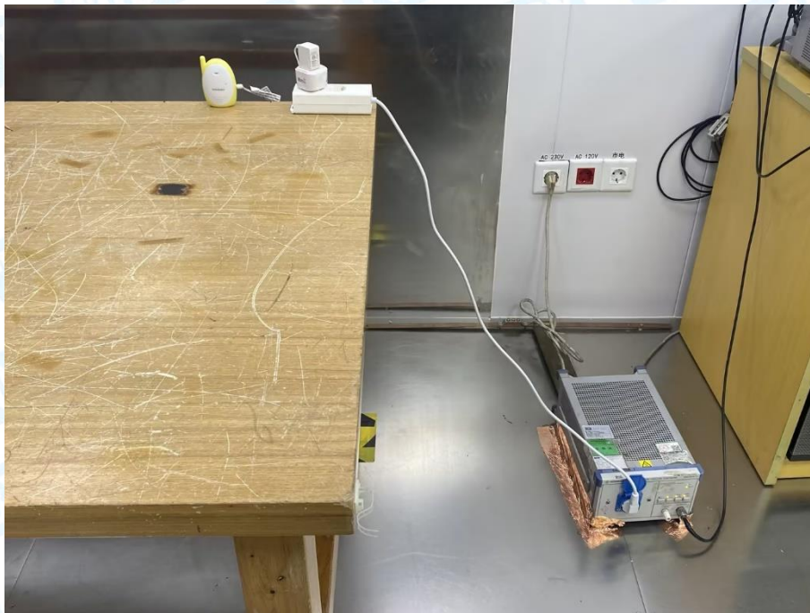
Photo of Setup for Conducted Emission
