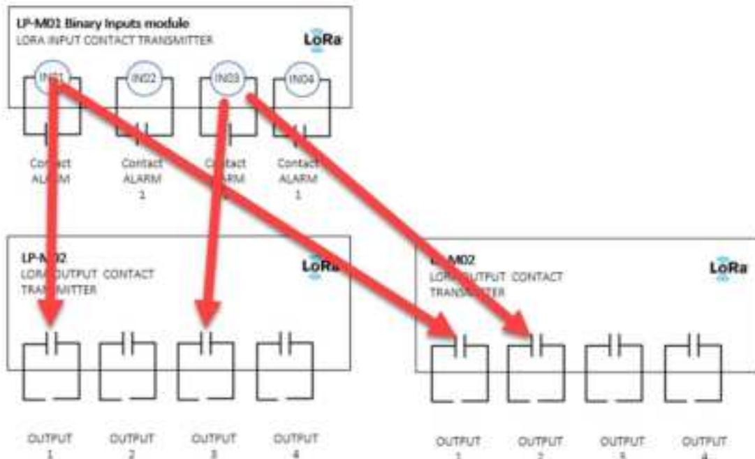
Figure 4.4 LP- M01input bundled to multiple M03
