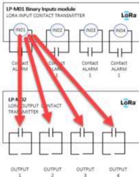
Figure 4.3 LP- M01input to multiple M03 output
