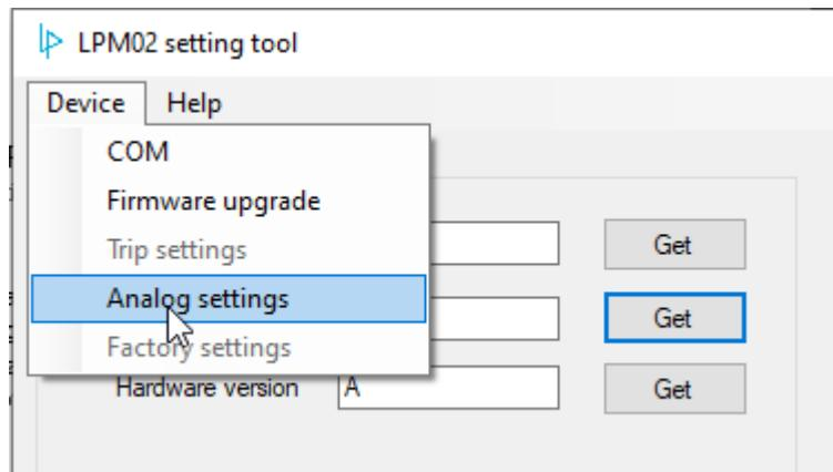
Figure 7.18 LP-M03 Setting Tool Analog Input setup select
