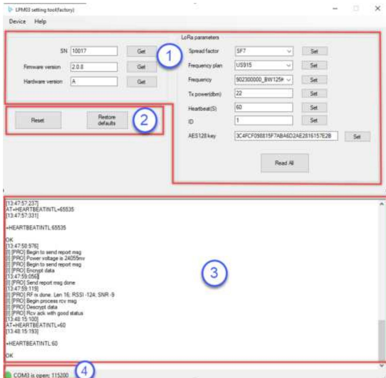
Figure 7.4 LP-M03 Setting Tool Interface
