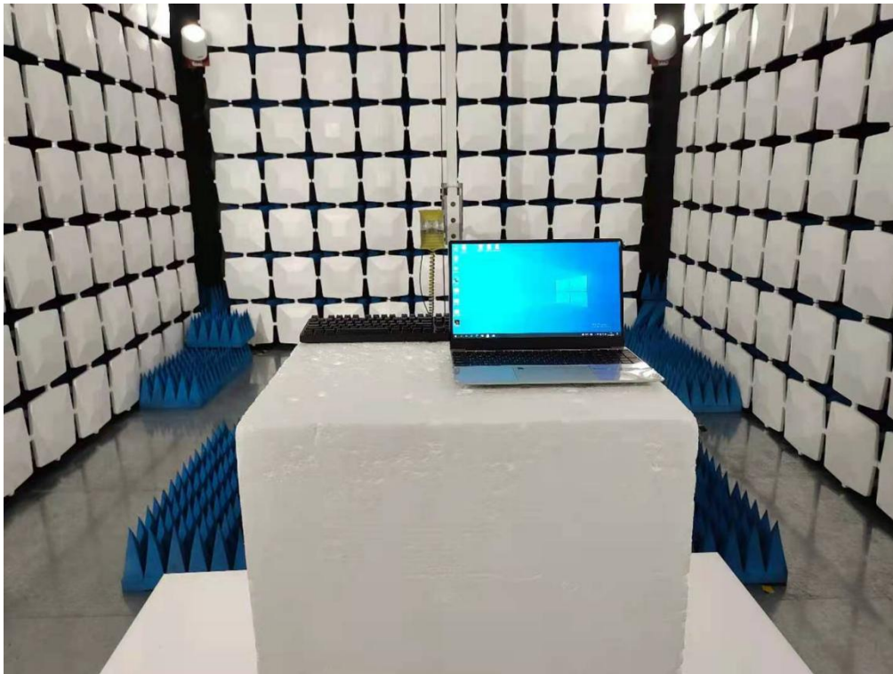
Above 1GHz for radiated emission test setup
