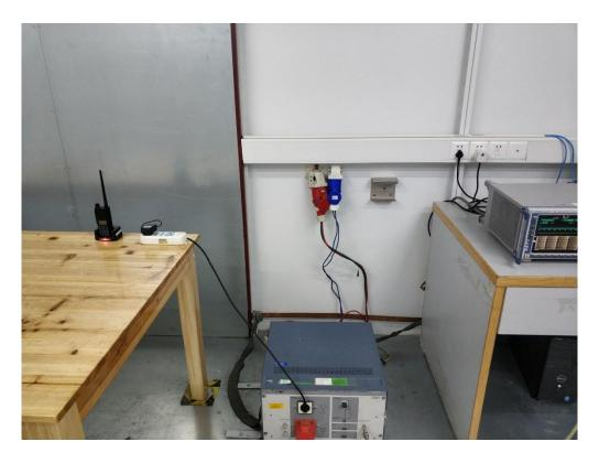
RADIATED EMISSION TEST SETUP-BELOW 1GHz
