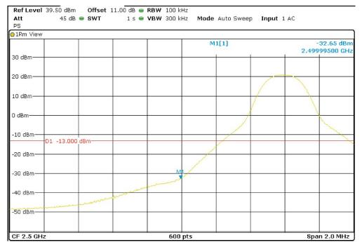
LTE QPSK MODULATION. RB = 1. Offset = Max. BW = 10 MHz
