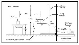
Radiated measurements > 1GHz
