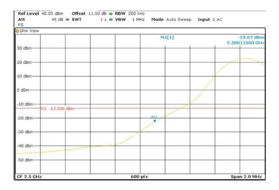
LTE QPSK MODULATION. RB = 1. Offset = Max. BW = 15 MHz
