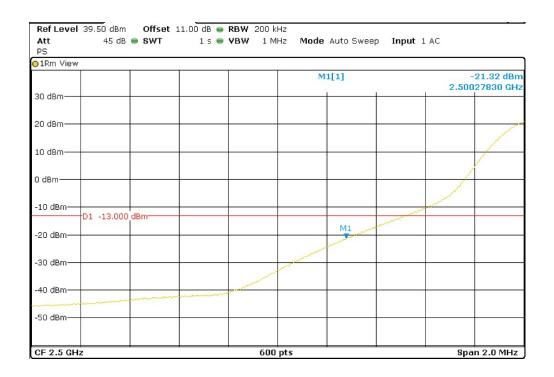
LTE QPSK MODULATION. RB = 1. Offset = Max. BW = 20 MHz
