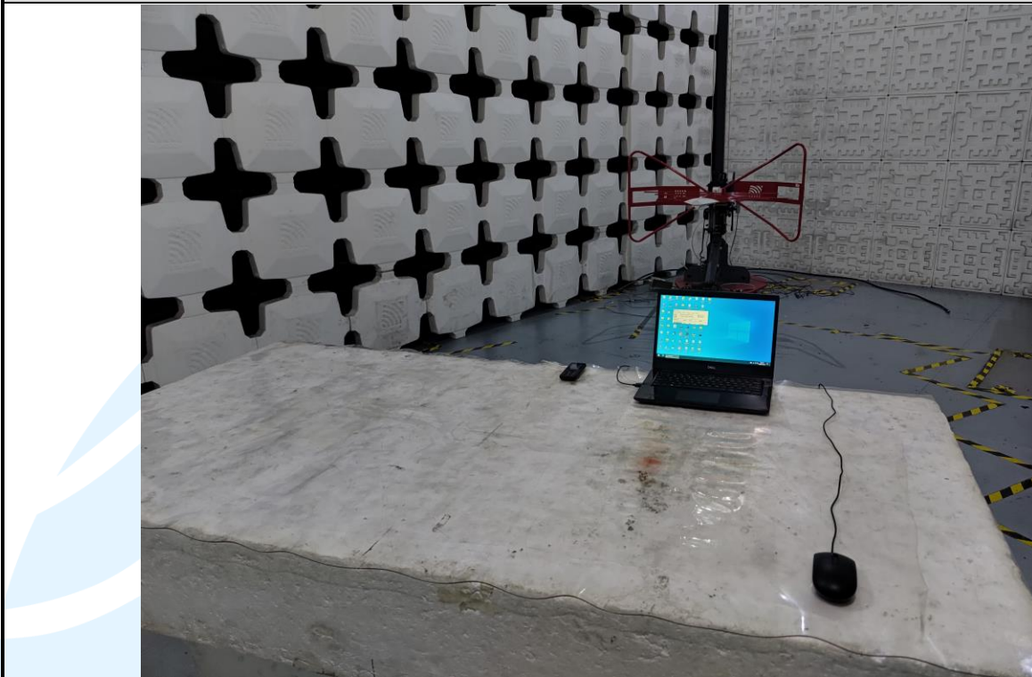
Radiated emission Test Setup-1 (30 MHz~1 GHz)
