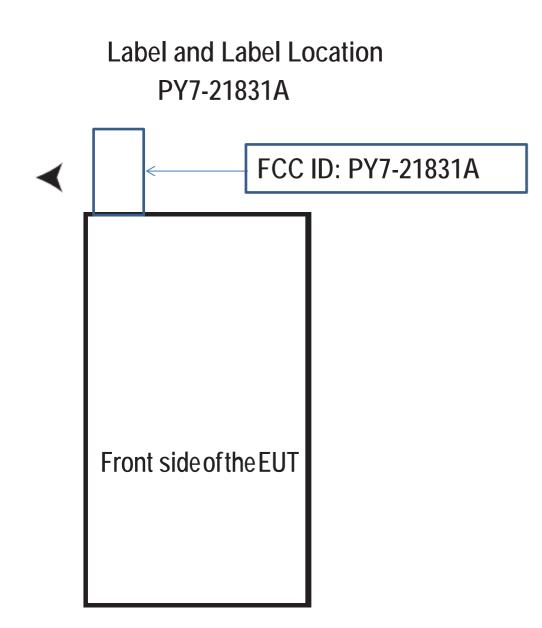
The FCC ID is not on the exterior of the device but labelling meets the conditions allowed in KDB 784748 for the label to be placed in a user accessible area:
