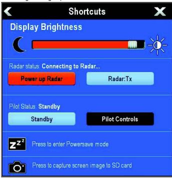
Multiple brightness groups can be configured. This can reflect the physical location of the units on your vessel if required. For example, the units at your helm can be set to one group, and the units on the flybridge can be set to a different group. In this example, any brightness adjustments made to a unit at the helm would be automatically reflected in the other units at the helm but not on the flybridge.
