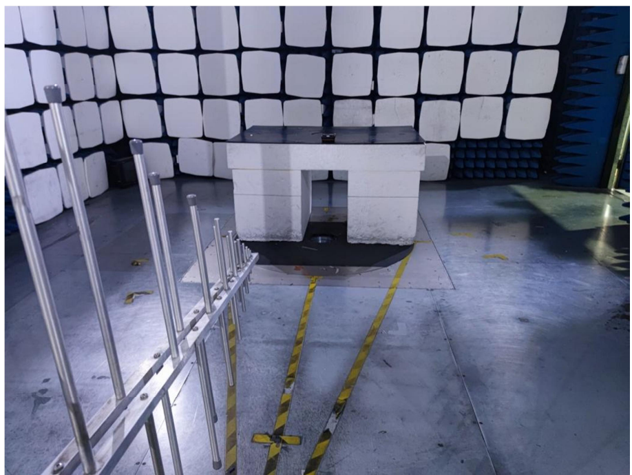
Radiation Emission Test Setup (30MHz to 1GHz)
