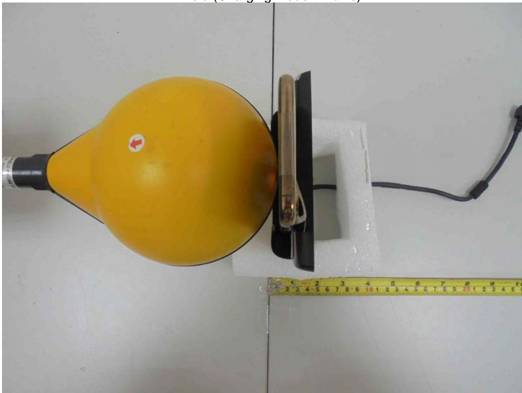
H-Field (Charging Mode - Z-axis)
