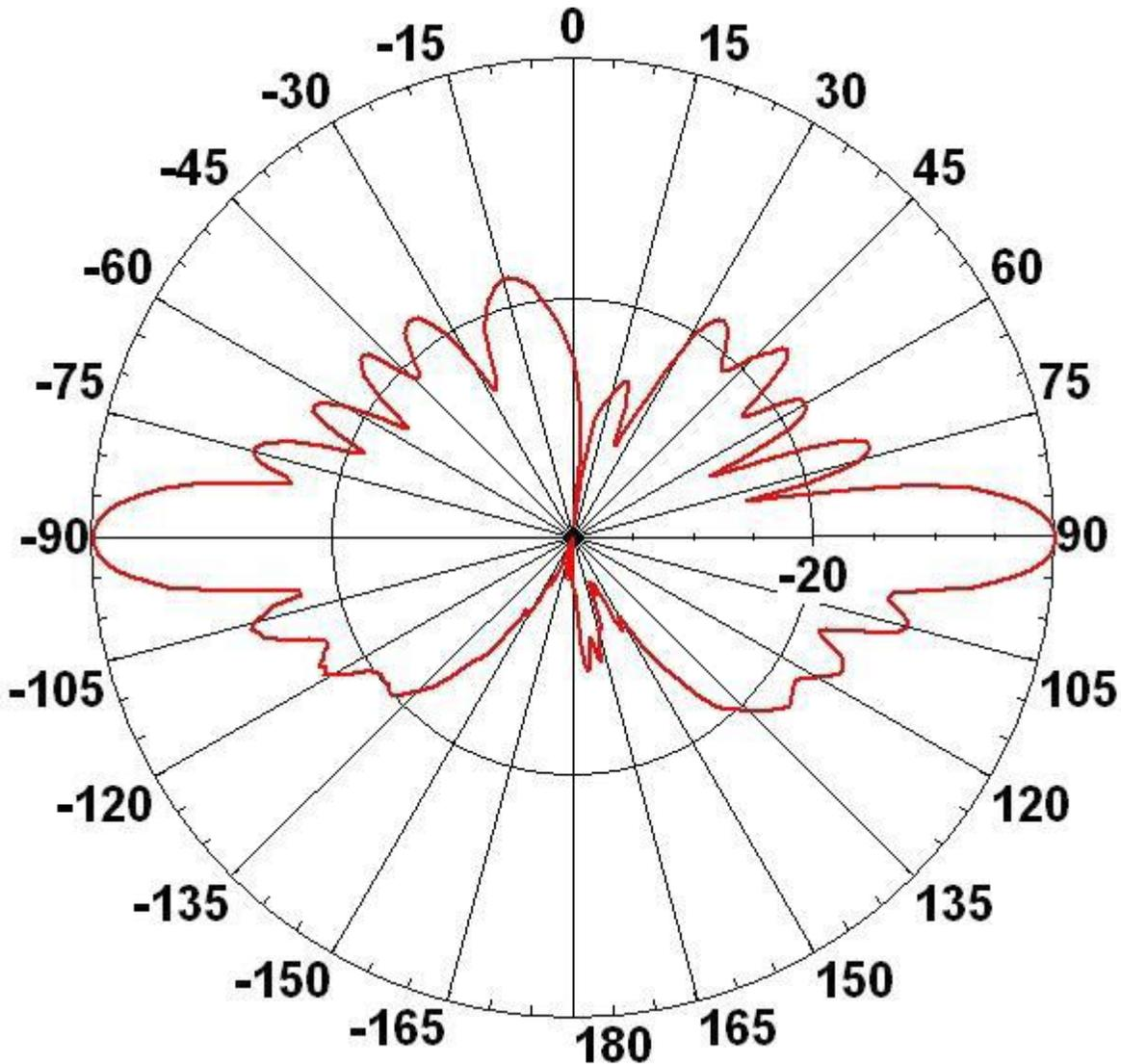
**Elevation Compliance Panel Antenna (24 dBi) PA58-24-ANT**
