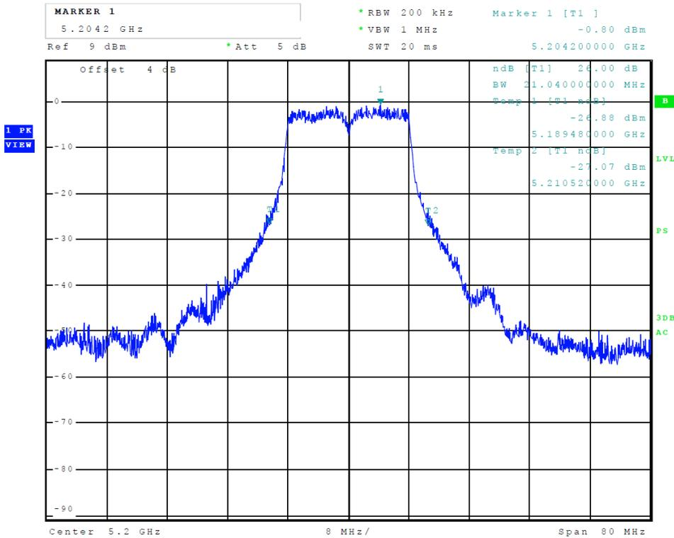
Figure 17 Plot of Transmitter Emissions (Chain 0, 5150-5250 MHz Band, 802.11a, 26 dB OBW)
