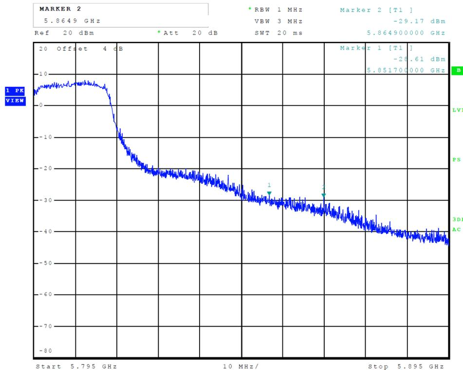
Figure 34 Plot of Transmitter High Band Edge (Chain 1, 5725-5850 MHz Band, 802.11n40)
