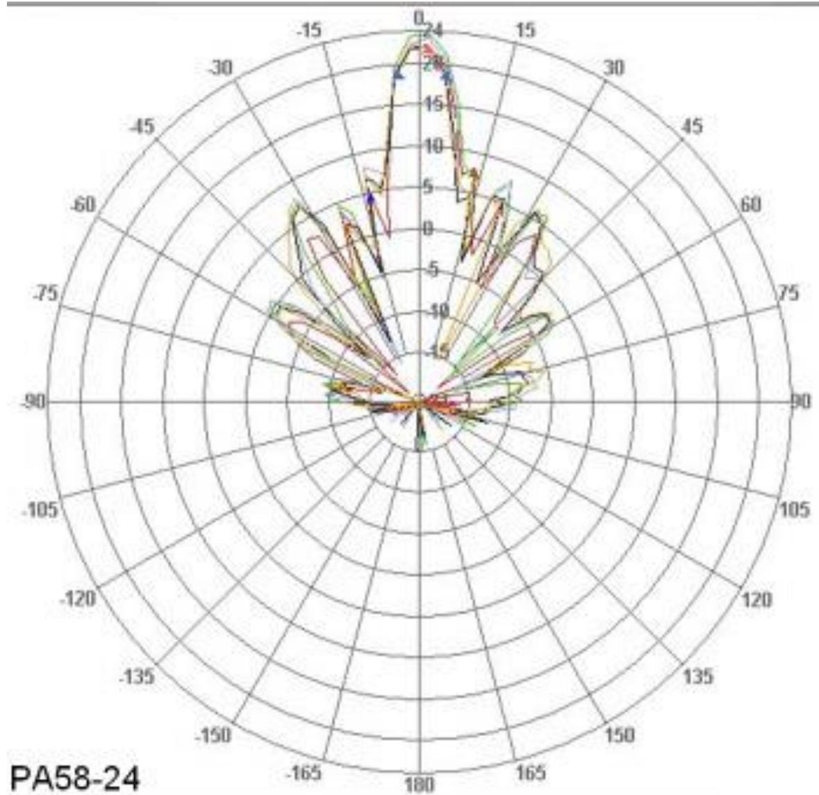
**Elevation Compliance Dish Antenna (32 dBi) HDDA5W-32-DP2**
