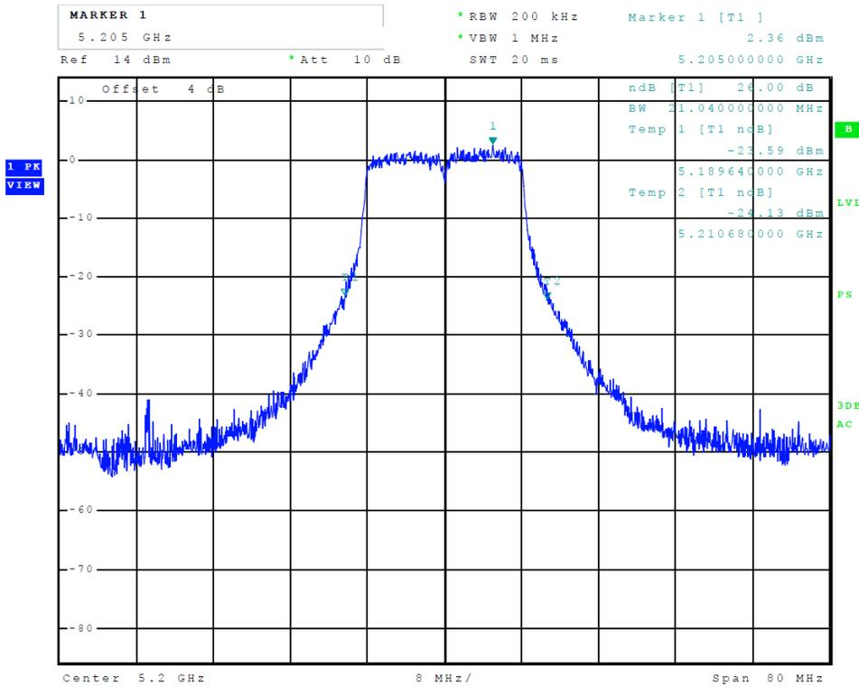
Figure 18 Plot of Transmitter Emissions (Chain 1, 5150-5250 MHz Band, 802.11a, 26 dB OBW)
