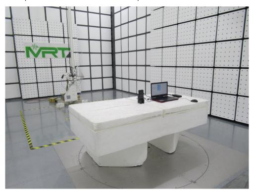
Description: Radiated Emission Test Setup for 1GHz~18GHz
