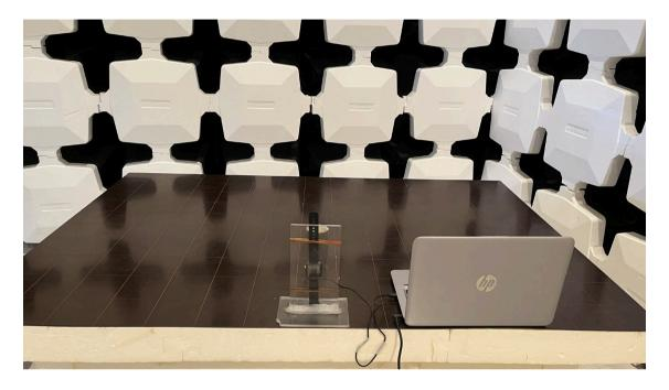
The EUT is placed in the center of the turntable
