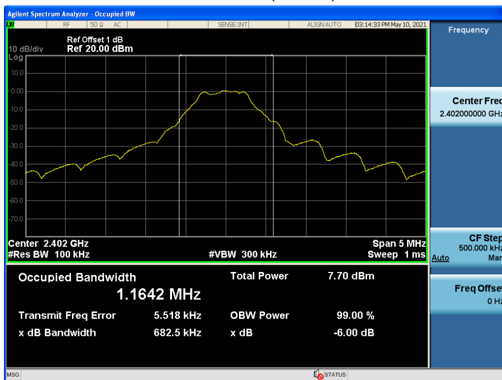
6dB Occupied Bandwidth Mode 1 / CH37 (2402MHz)
