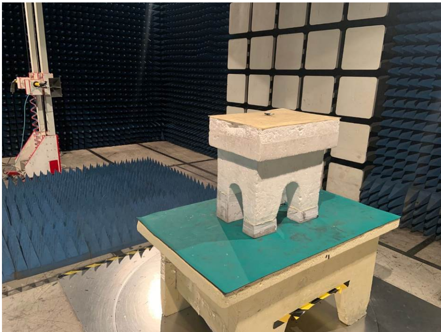
Spurious Emission Test Setup (Above 1GHz)
