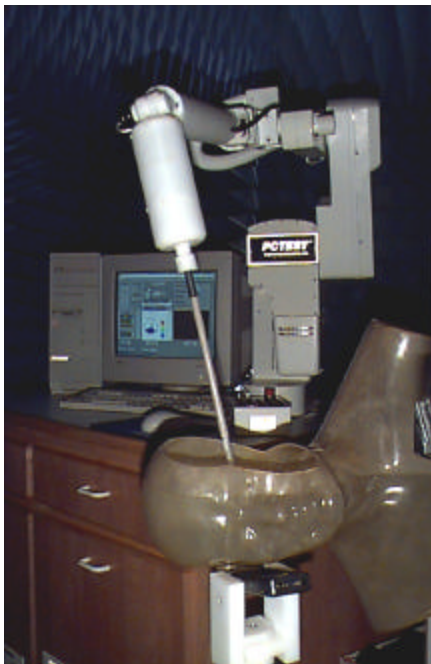
Figure 5. Photograph of the Probe and the Phantom
