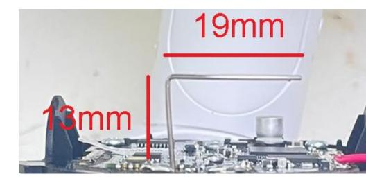
Figure 1 Physical dimension (mm)
