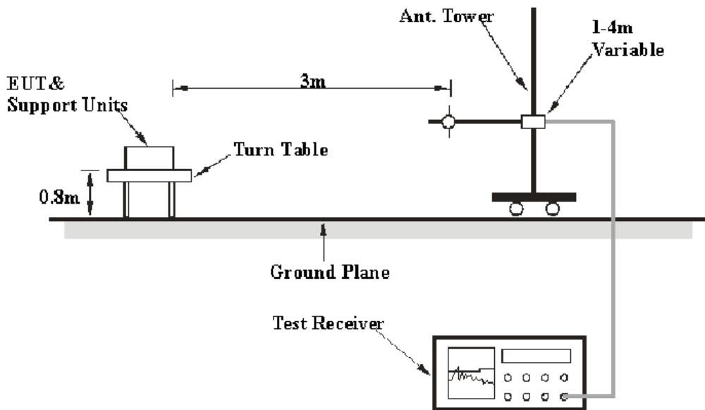
The radiated emission tests were performed in the 3-meter chamber a test site, using the setup accordance with the ANSI C63.10-2013.
