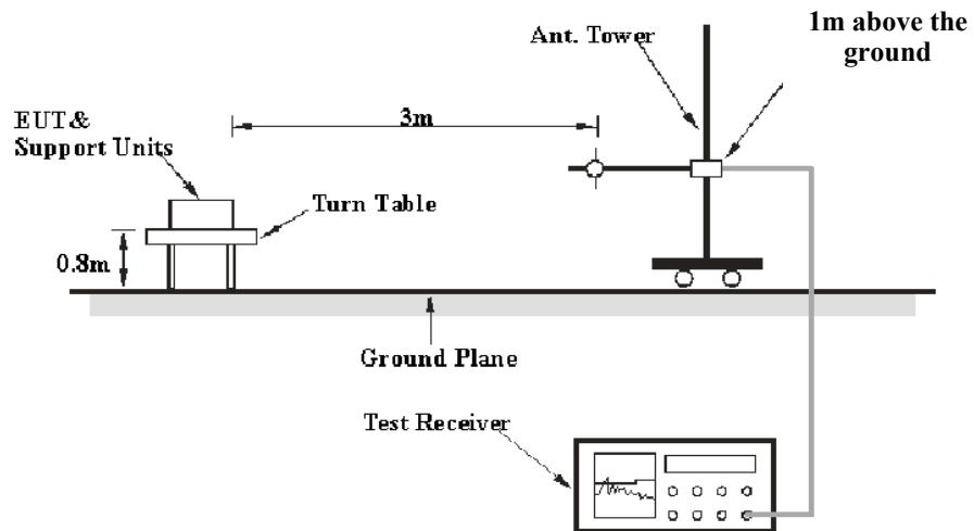
Note: Antenna is set up at 1m during test for below 30MHz.
