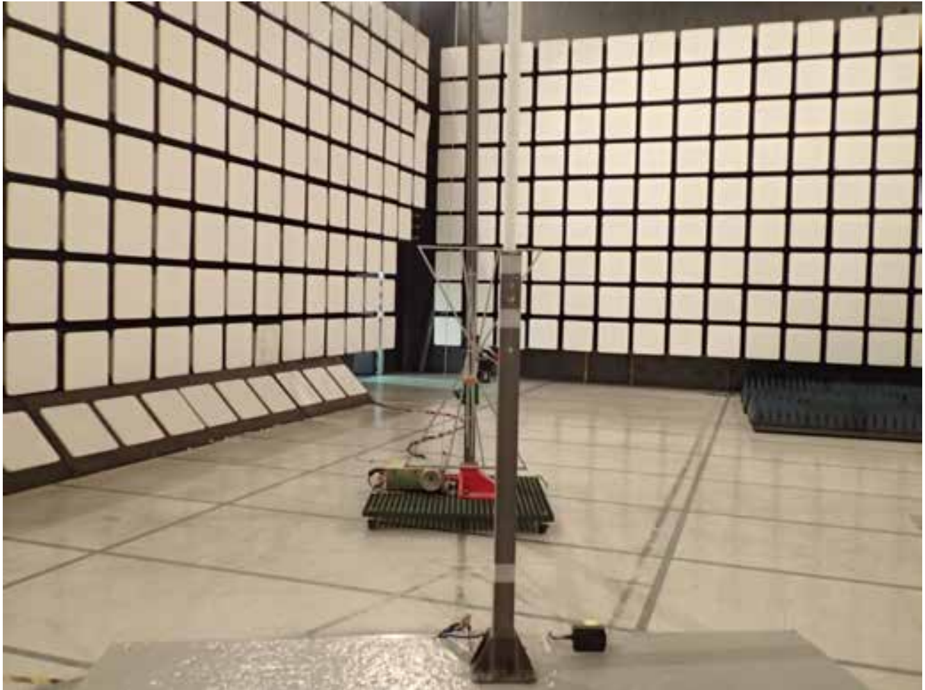
Radiated Emissions @ 3 m EUT with 8.15 dBi Omni Directional Antenna, Orthogonal Position 1
