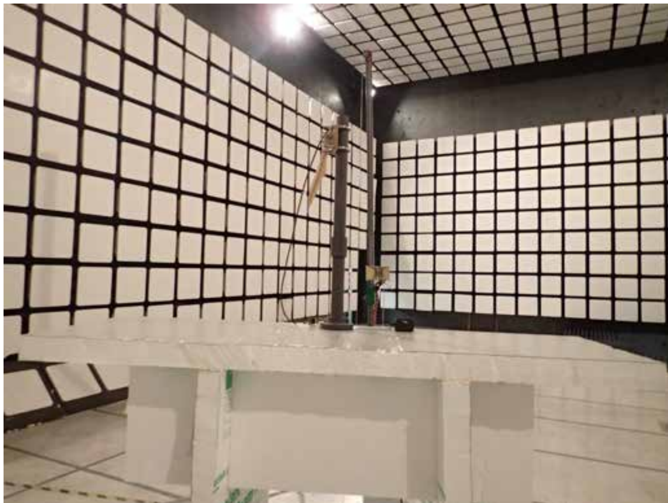
Radiated Emissions @ 3 m EUT with 13.15 dBi Yagi Antenna, Orthogonal Position 2
