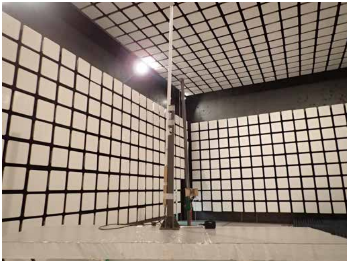
Radiated Emissions @ 3 m EUT with 8.15 dBi Omni Directional Antenna, Orthogonal Position 2
