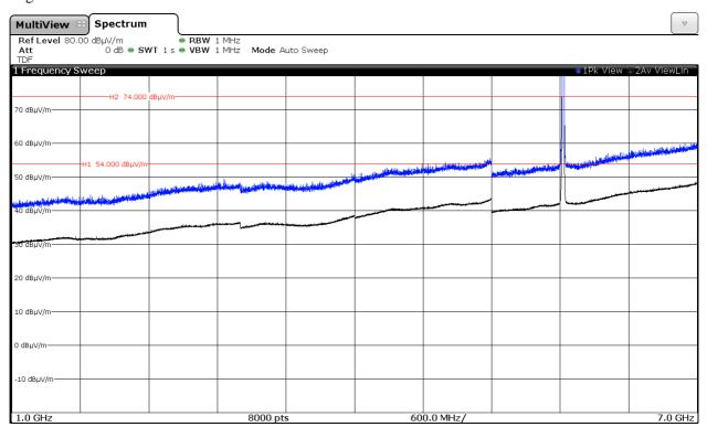
Note: The peak above the limit is the carrier frequency.
