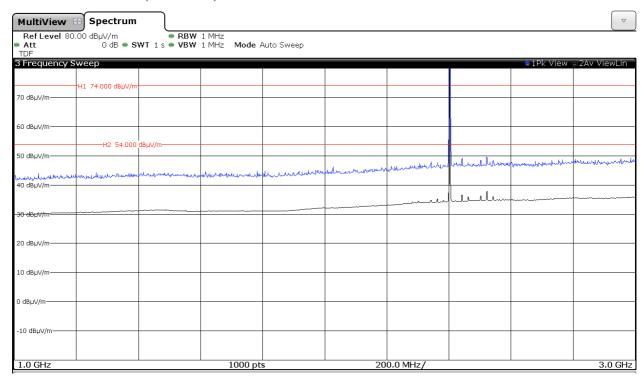
Note: The peak shown in the plot above the limit is the carrier frequency.
