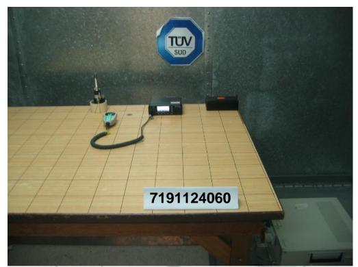
Conducted Emissions Test Setup (Front View)
