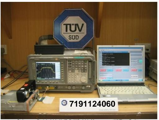
Spectrum Bandwidth (6dB Bandwidth Measurement) Test Setup
