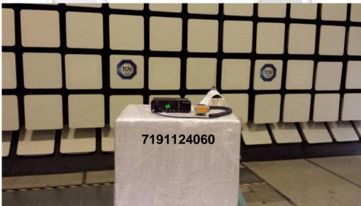
Band Edge Compliance (Radiated) Test Setup
