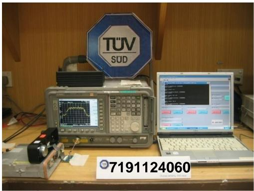
Band Edge Compliance (Conducted) Test Setup
