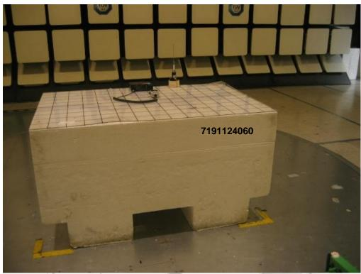
Radiated Emissions Test Setup (Front View)
