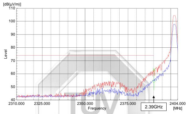
Plot 35 - Peak Plot at Lower Band Edge at 2.4000GHz
