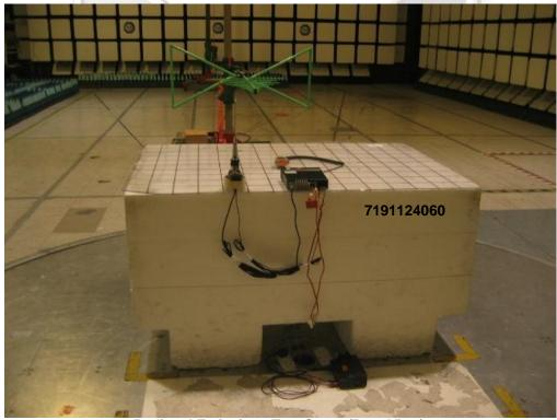
Radiated Emissions Test Setup (Rear View)
