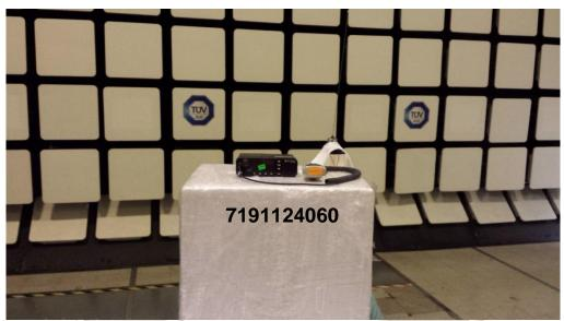
Radiated Emissions Test Setup (Front View)
