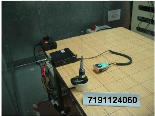
Conducted Emissions Test Setup (Rear View)
