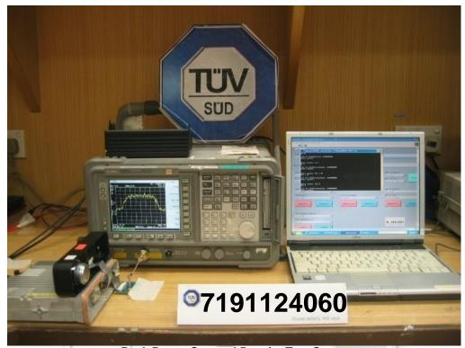
**Peak Power Spectral Density Test Setup**
