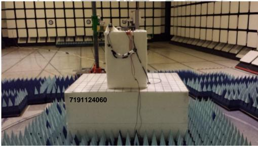
Radiated Emissions Test Setup (Rear View)
