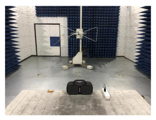
RADIATED EMISSION TEST SETUP ABOVE 1GHZ
