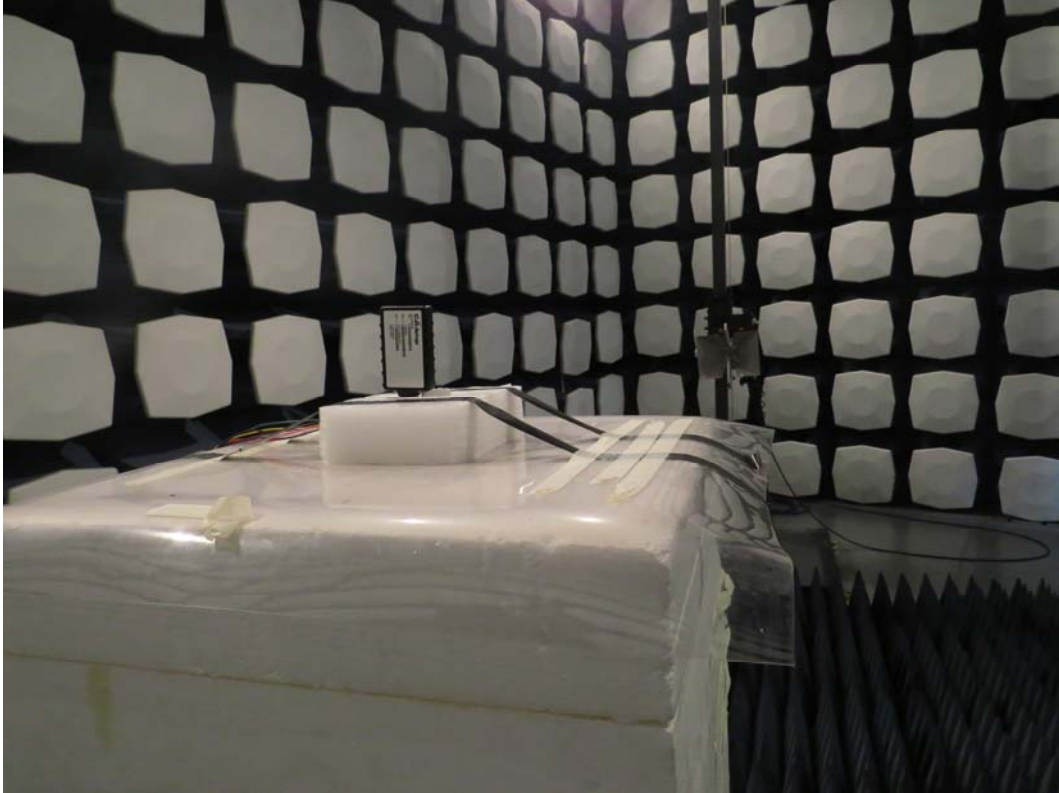
Picture 2: Radiated Spurious Emissions Test setup
