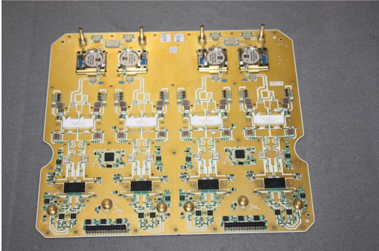
**Top View of CU Board with Shield Removed**
