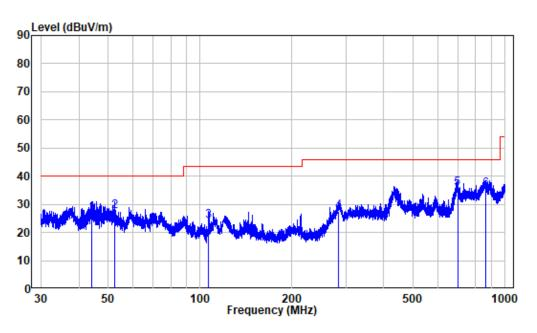
Site : chamber Condition: 3m VERTICAL Test Mode: BT Transmitting Power : AC 120V/60HZ
