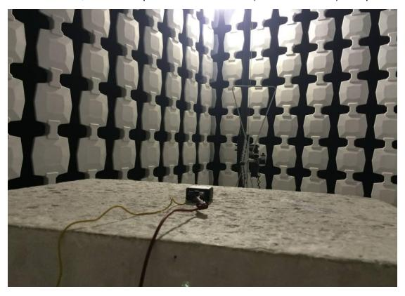
EIRP Test, Radiated Spurious Measurement (Above 1GHz) Setup
