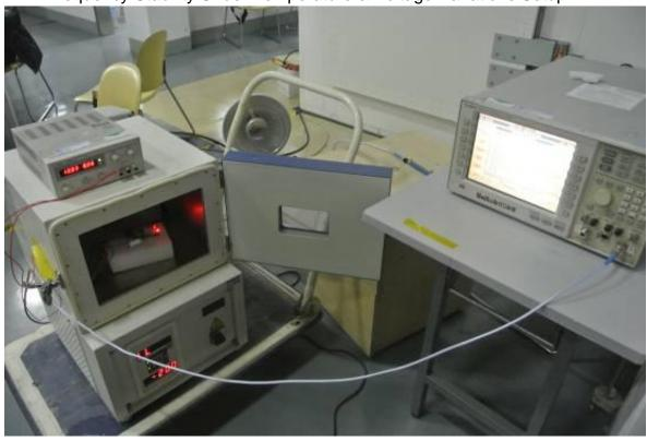
Radiated Spurious Measurement(below 30MHz) Setup
