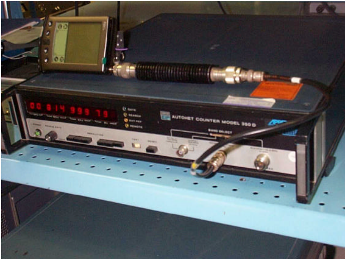
Palm V and Wavenet DWV 100D PDA Wireless Modem tested for Frequency Stability at Power Variation
