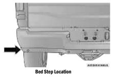
To extend the bed step, place your foot on the protruding foot tab located on the left edge of the bed step, and push rearward. A small amount of force will release the spring load and extend the bed step out and away from the tailgate.
