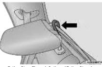
Tether Strap Through Outboard Tether Strap Loop
