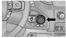
**Electronic Transmission Gear Selector**
