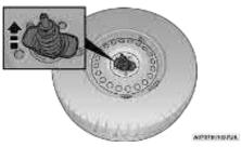
**Reinstalling The Retainer**
