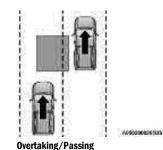
The BSM system is designed not to issue an alert on stationary objects such as guardrails, posts, walls, foliage, berms, snow banks, car washes etc. However, occasionally the system may alert on such objects. This is normal operation and your vehicle does not require service. The BSM system will not alert you of objects that are traveling in the opposite direction of the vehicle in adjacent lanes  $\[colored]$  page 458.
