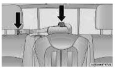
Tether Strap Through Center Tether Strap Loop And Attached To Outboard Tether Strap Loop
