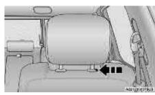
**Head Restraint Adjustment Button Location**
