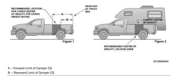
When the truck is used to carry a slide-in camper, the total cargo load of the truck consists of the manufacturer's camper weight figure, the weight of installed additional camper equipment not included in the manufacturer's camper weight figure, the weight of camper cargo, and the weight of passengers in the camper. The total cargo load should not exceed the truck's cargo weight rating and the camper's CG should fall within the truck's recommended CG zone when installed.
