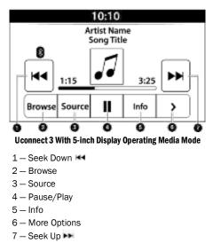
Media Mode is entered by pushing the MEDIA button located on the faceplate.
