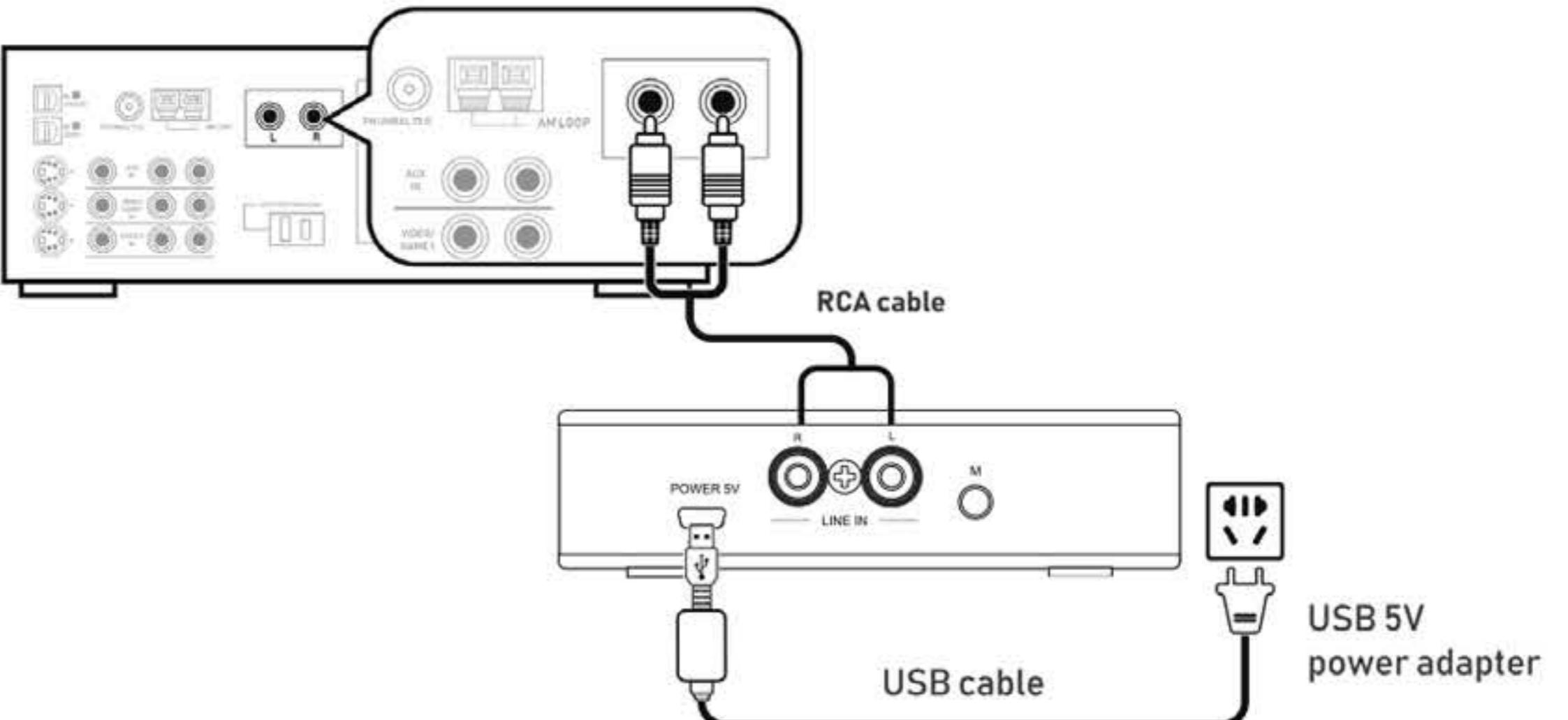
**Step 1** - Use the supplied (d) RCA cable to connect the Subwoofer Pre-Out or LFE output of your AV receiver and to the (a) WSK SUB wireless transmitter Audio Input. *You can leave right RCA plug unconnected if you are connecting to a subwoofer as mono signal*
