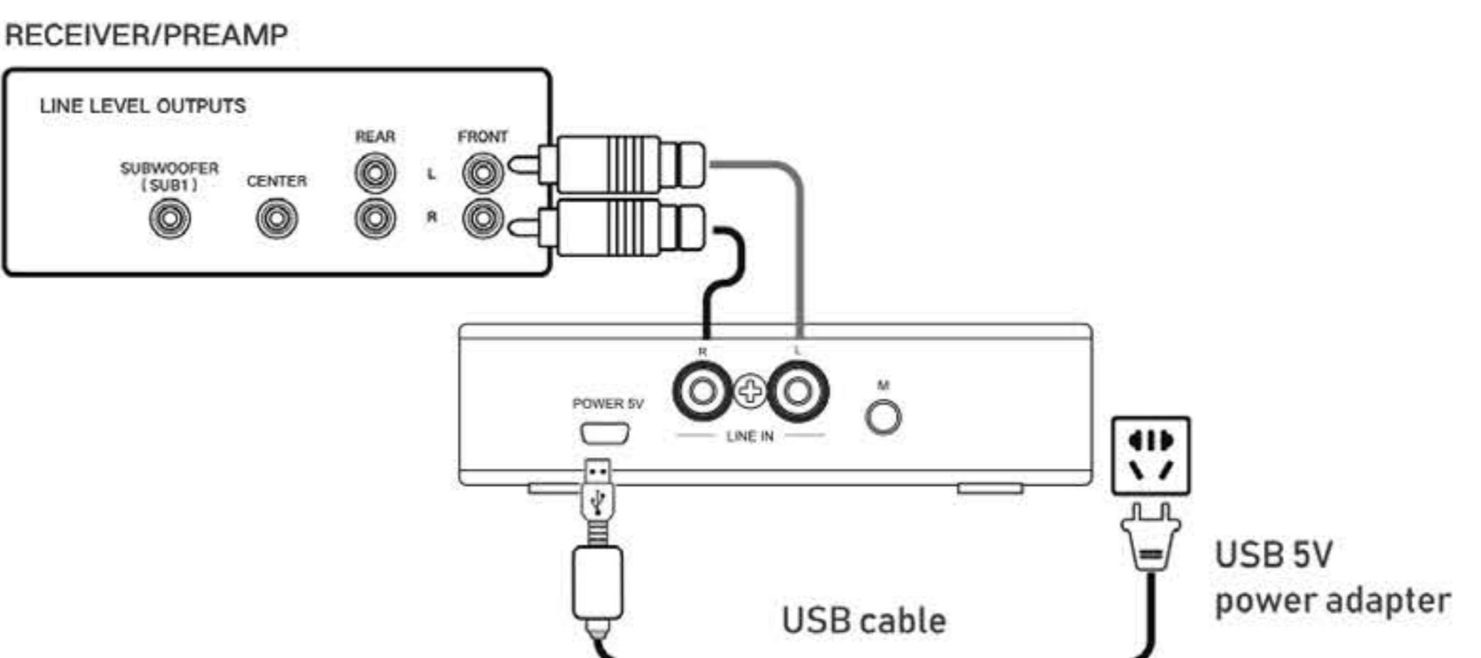
**Step 1** - Use the supplied (d) RCA cable to connector the 2 channel stereo pre-amplifier's L/R line level Pre-Outs to (a) WSK SUB wireless transmitter L/R input
