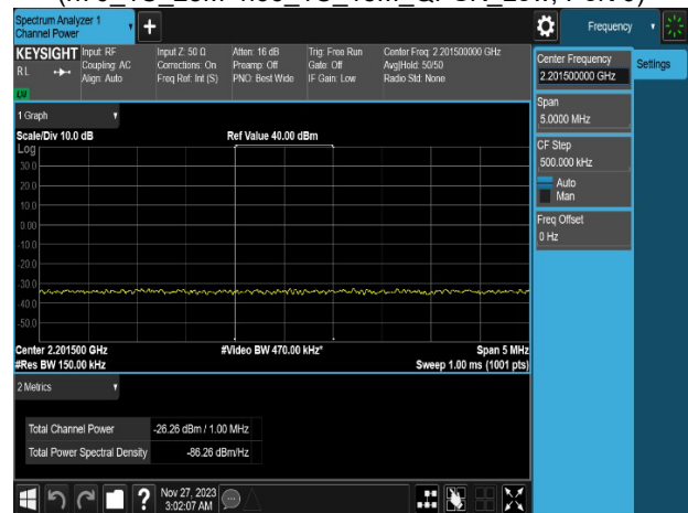
Plot 8-114. Conducted Spurious Emission Plot 2.201 GHz to 2.202 GHz (n70_1C_25M+n66_1C_15M_QPSK_Low, Port 0)
