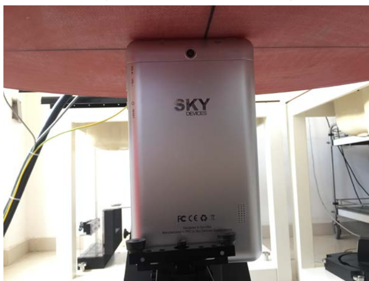
Test Position 4 - Body-worn, the top side of the EUT towards ground (The distance was 0mm)
