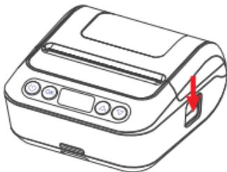
2. Install the paper roll as shown in the figure below.
