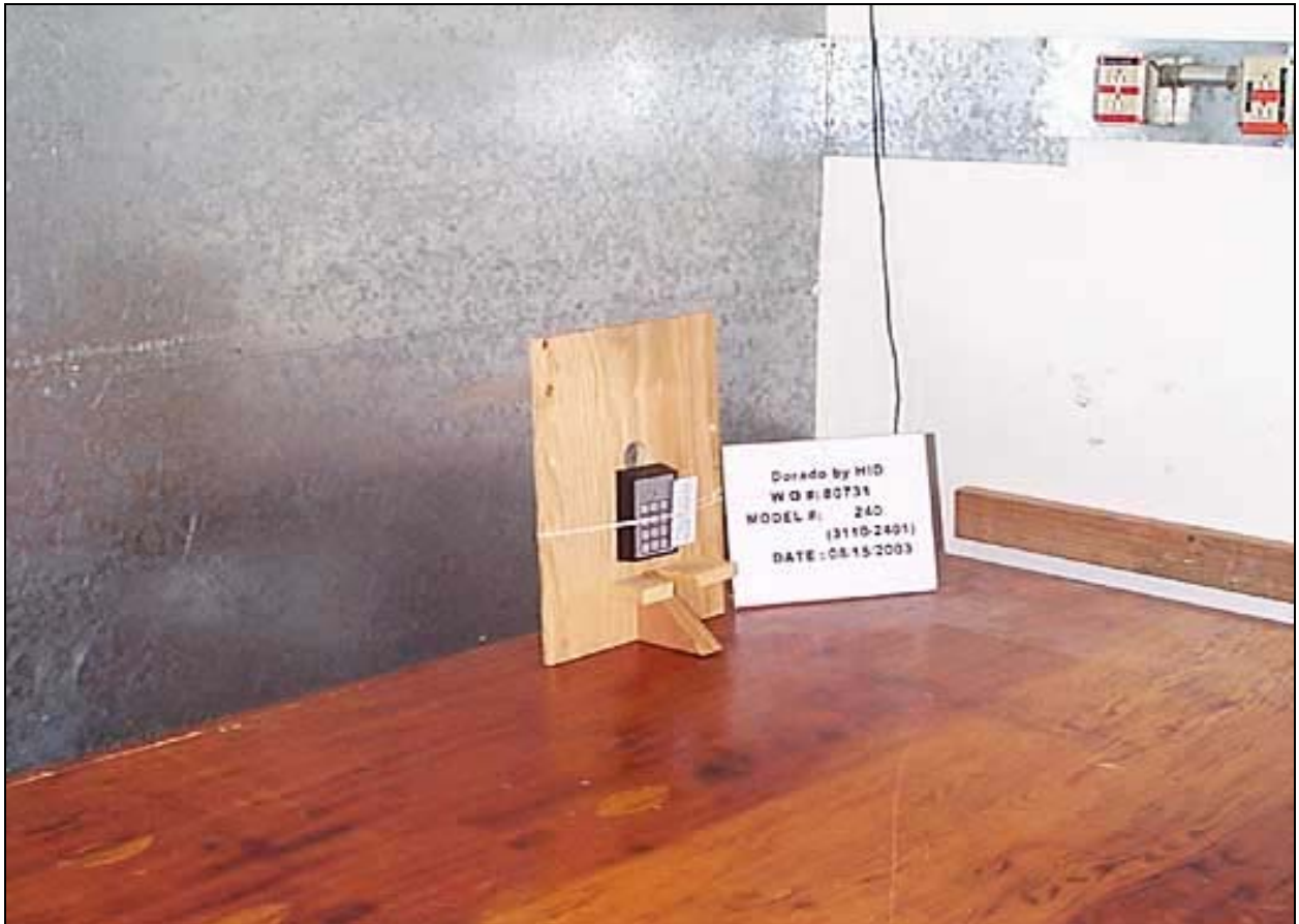
Mains Conducted Emissions - Front View
