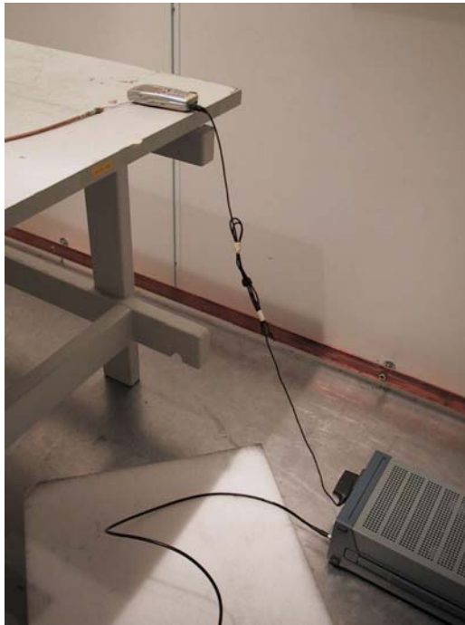
Picture 1: AC-power line conducted emissions test setup
