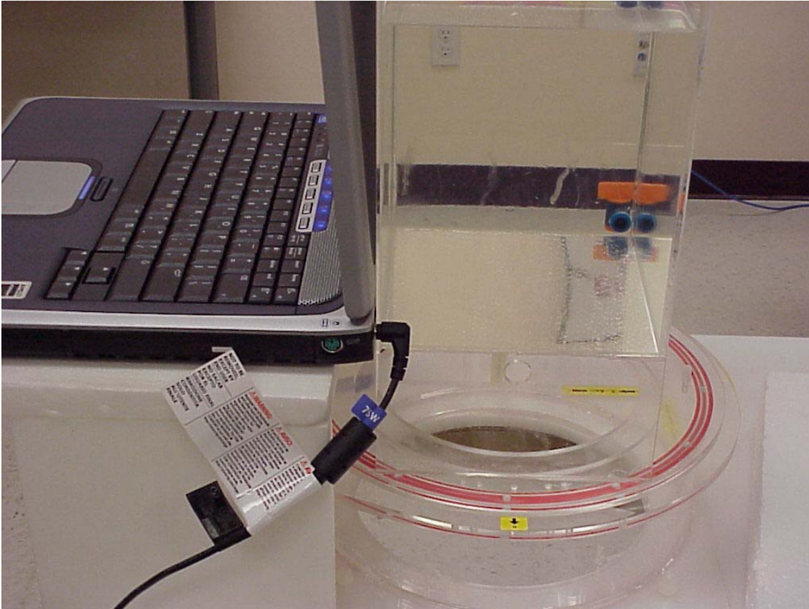
Photo 7. Right Antenna Rear Bystander Position
