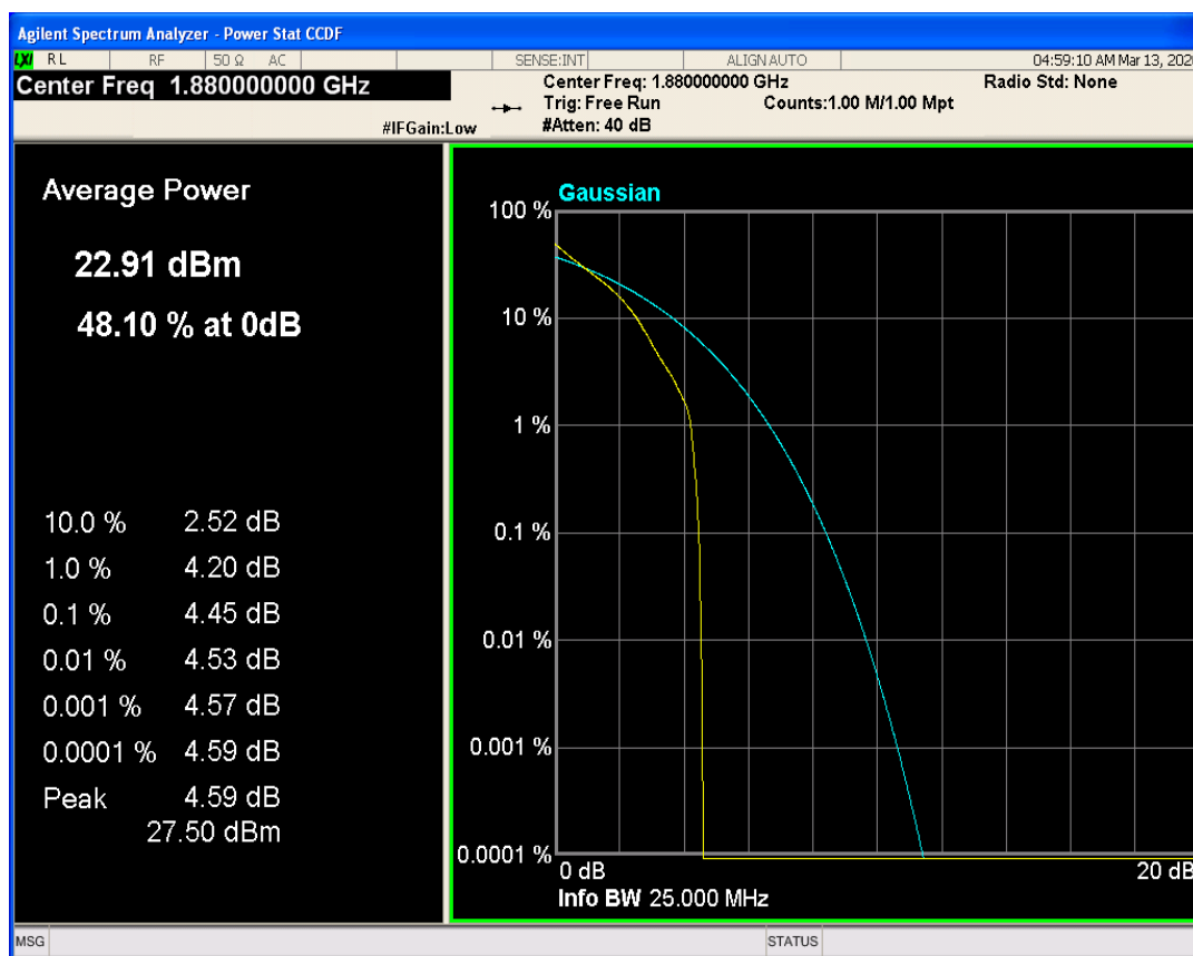
LTE Band2 QAM16 BW=1.4MHz Channel=18900 RB Size=1 Position=#0
