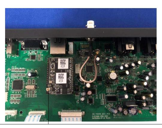
This is Wi-Fi module, But closed Wi-Fi function on this product, only used the RJ45 ethernet function. The Wi-Fi function has been closed, and this ipex connector have not used.
