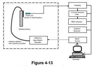
Audio Magnetic Field Test Setup
