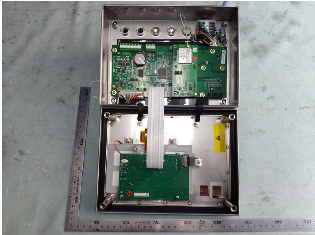
FIGURE 9 WEIGHING TERMINAL (M/N: IND256X) COVER REMOVED
