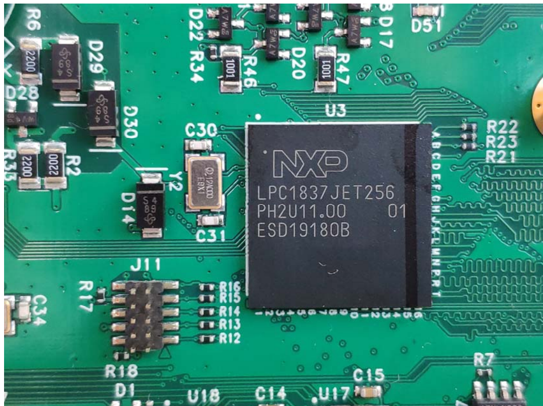
FIGURE 15 WEIGHING TERMINAL (M/N: IND256x) CRYSTAL & CHIP ON MAIN BOARD
