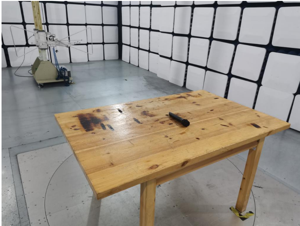
Photo of Radiation Emission Test
