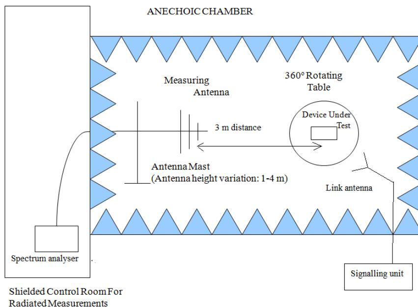
Radiated measurements between 1 GHz and 18 GHz.
