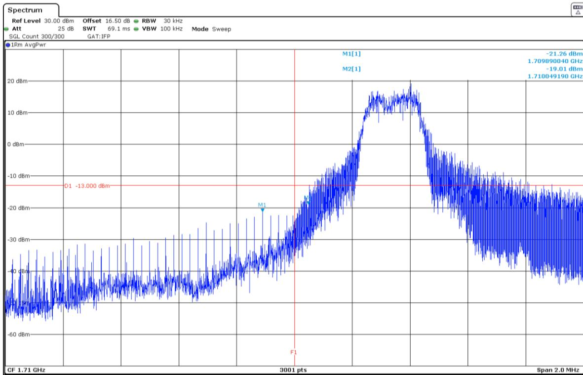
QPSK. Nominal Bandwidth 5 MHz. RB Size 1, RB Offset Max. Narrow band = 3. High Block Edge:
