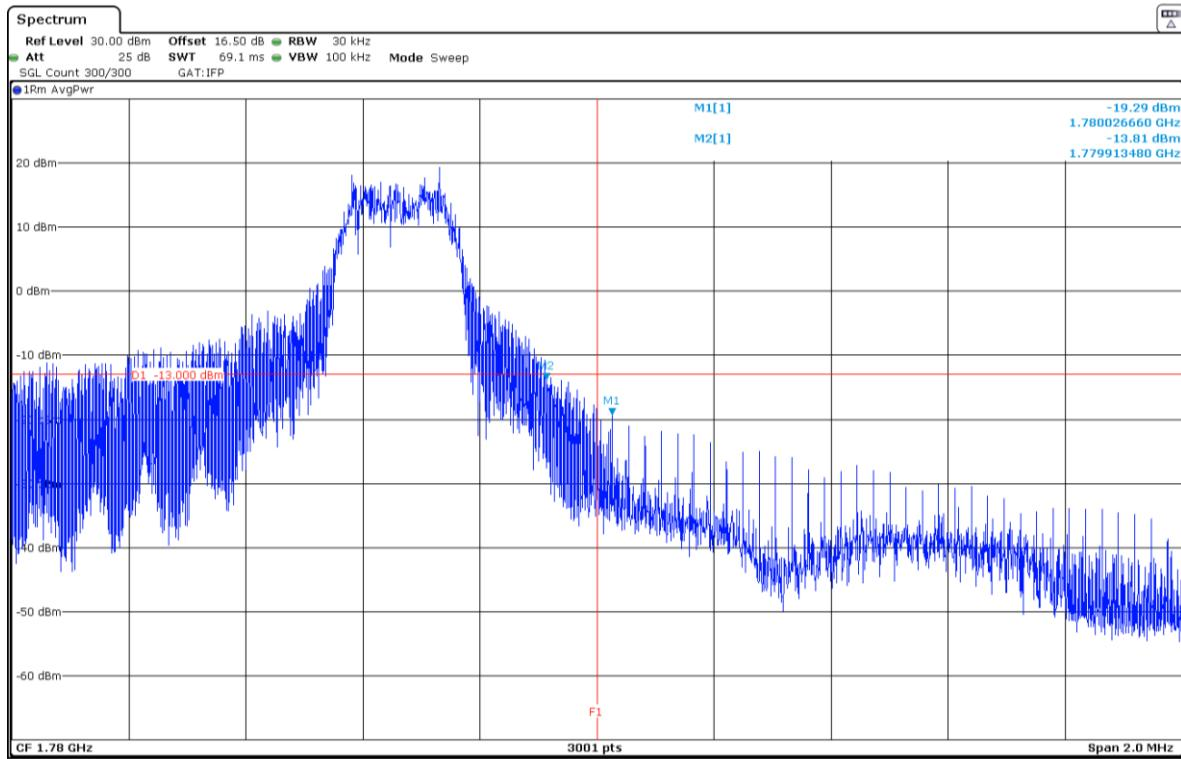
QPSK. Nominal Bandwidth 5 MHz. RB Size All, RB Offset 0. Narrow band = 0. Low Block Edge:
