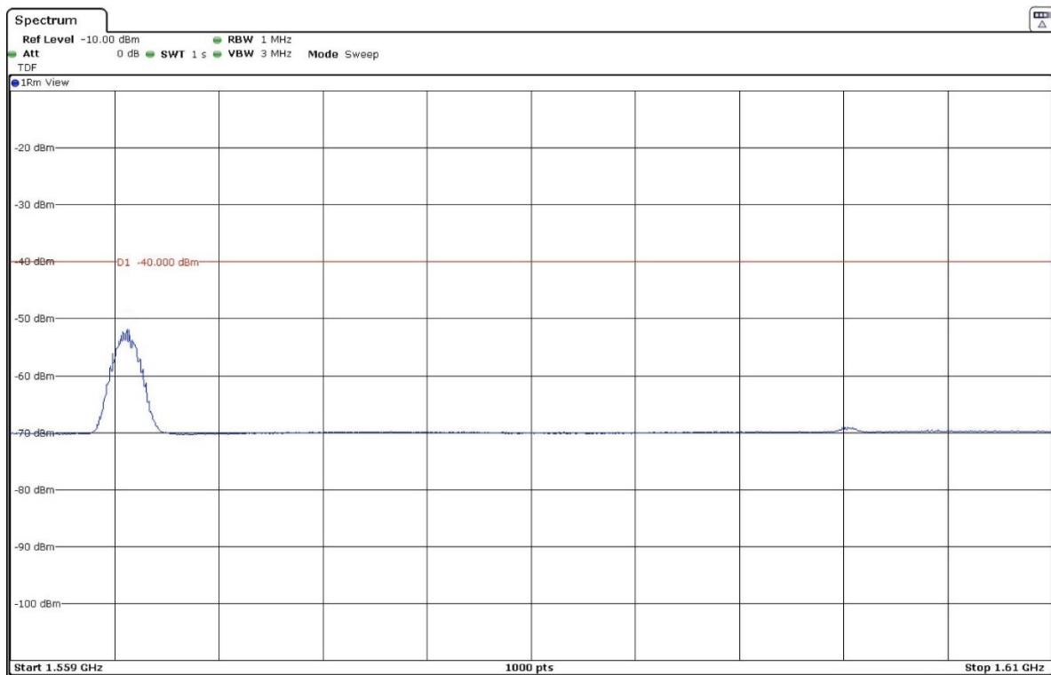
LTE Band 66. QPSK. Nominal Bandwidth 20 MHz. RB Size 1, RB Offset 0. Narrow band = 0, Position 1.
