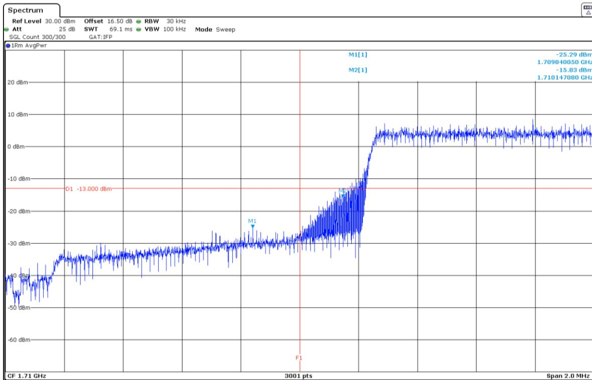
QPSK. Nominal Bandwidth 5 MHz. RB Size All, RB Offset 0. Narrow band = 3. High Block Edge:
