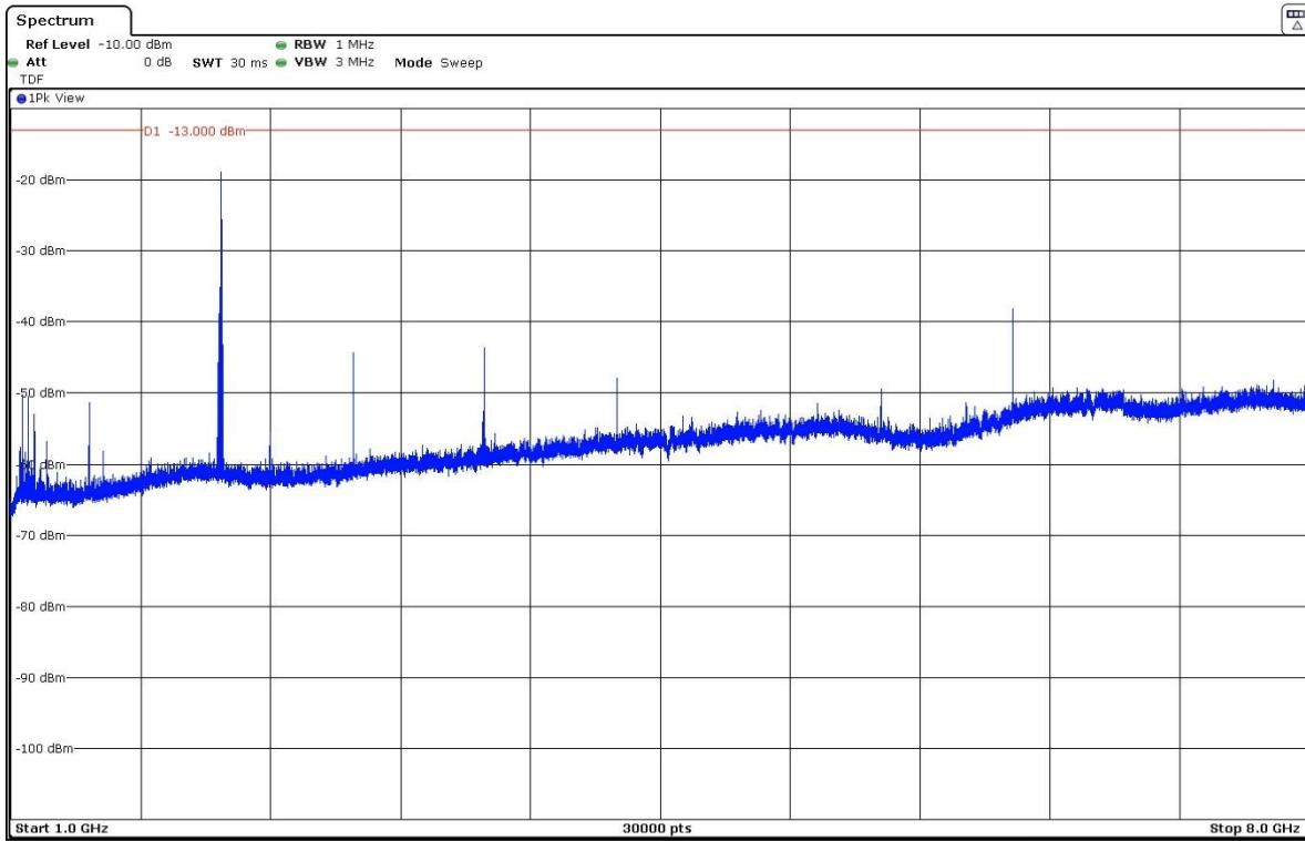
LTE Band 13. QPSK. Nominal Bandwidth 5 MHz. RB Size 1, RB Offset 0. Narrow band = 0, Position 1.
