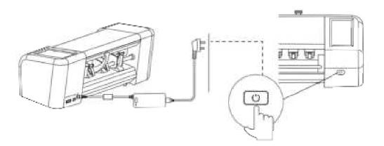
Connect the power cord to the adapter and then connect the power cord to the power socket. To ensure the normal operation of the device, please use 100-240 volts AC power; Connect the adapter to the power interface of the device; Install the blade kit on the knife holder to ensure it is fixed correctly. After connecting, press [Power Switch] to start the device.
